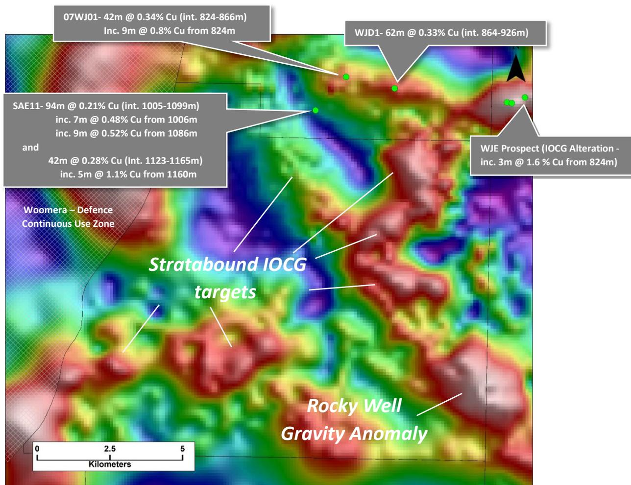
Figure 2 - Significant historical IOCG copper intersections adjacent to Petratherm’s Woomera Licence Area (EL 6707) overlain on a Residual Gravity Image. High gravity areas (red-white zones) may indicate zones of stratabound style and breccia style IOCG mineralisation.
