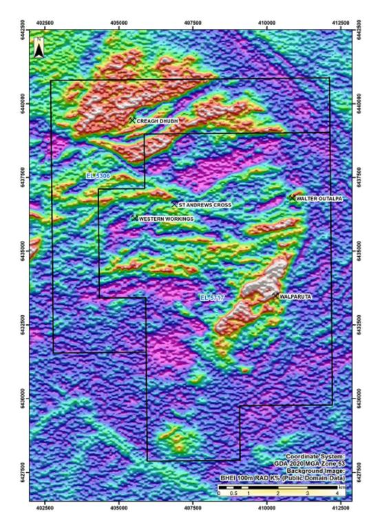
Figure 11: Walparuta project BHEI Radiometric Survey (100m) K % and prospect locations.
