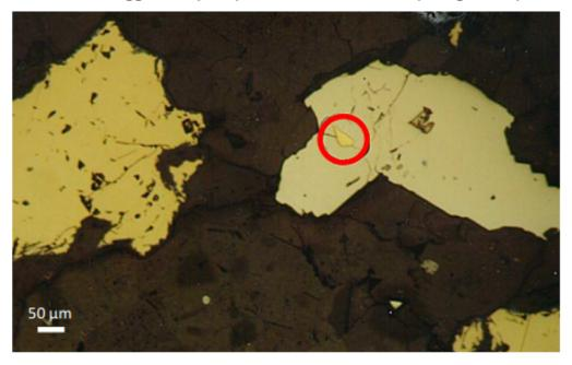
Figure 13: Photomicrograph from Walparuta Cu-Au Mine. Yellow Mineral = Chalcopyrite, White Mineral = Pyrite and Red Circle = Au (25x50µm) (Pontifex, 1990).
